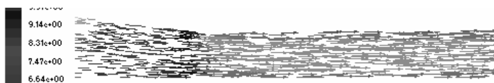
图 14 左线 2# 竖井排风联络风道铅垂面速度矢量图 Fig.14 Velocity vector graph of consecution duct for exhaust duct of 2# vertical shaft in left tunnel
