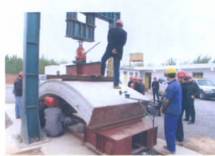
图 4 管片抗弯试验 Fig.4 Bending test of single segment
